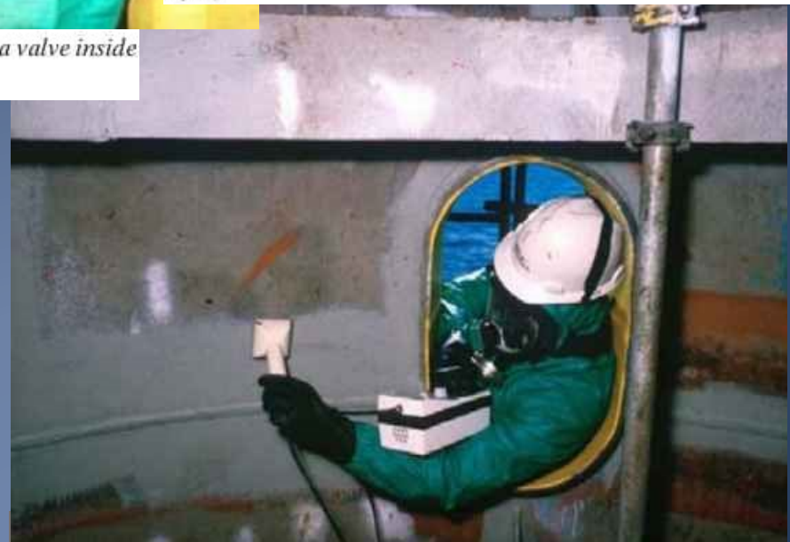
NORM contamination within a vessel being measured using a surface contamination measuring instrument (courtesy: National Radiological Protection Board,
